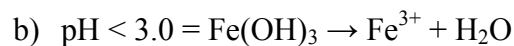
Fig. 5. – The precipitation of ferric hydroxide ( \text{Fe}(\text{OH})_3 ) and the production of ferric ions ( \text{Fe}^{3+} ) depending on pH.
