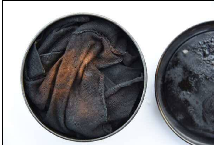
Figure 5.11: Char Cloth – Using the pyrolysis process, the cotton cloth is heated without oxygen. The lighter colored fabric is not yet fully processed. Source: author – [file:\FR-CharCloth03.jpg].
