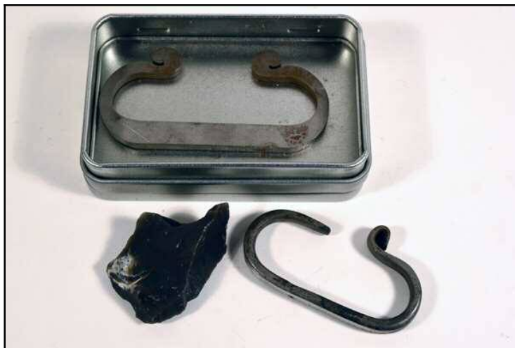
Figure 5.4: Flint and Steel – Striking the flint against the steel can send a spark which is burning steel with a temperature of 2,498°F. Source: author – [file:\FR-Flint&Steel05.jpg].
