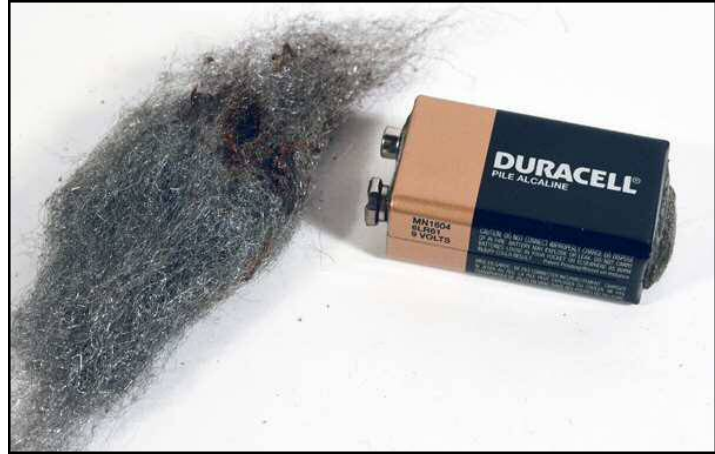
Figure 5.7: Battery and Steel Wool – The battery provides an electric current that shorts out and ignites the steel wool. Source: author – [file:\FR-Battery&SteelWool07.jpg].
