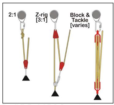
Figure 6.1: The Three Basic Hauling Systems – Source: rbk
