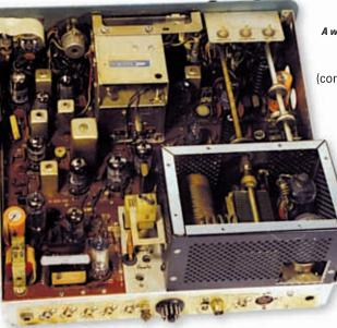
There were a few semiconductors used in the design and they were mostly diodes. The exception was the v.f.o. which employed an MPF105 field effect transistor (f.e.t.) as the oscillator (buffered by a 6AU6).
